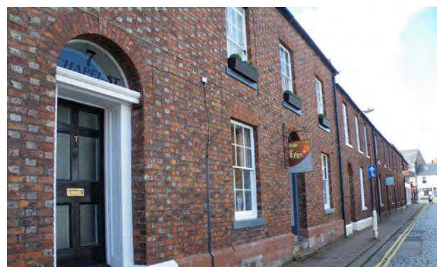
Fig 11. The 1820s Chapel Street - a red brick terrace with distinctive chequerboard brickwork.
