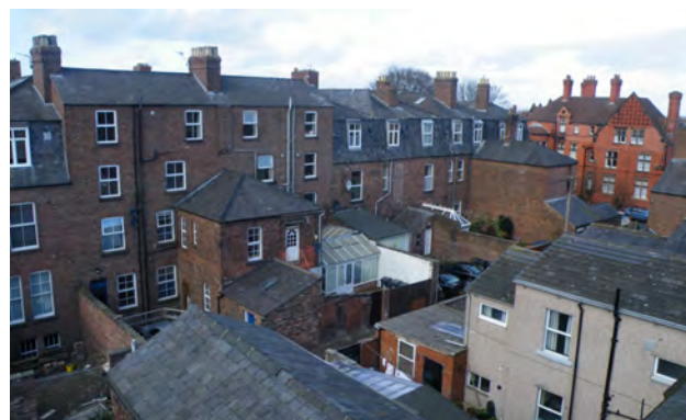
Fig 54. The roofscape of the CA is typically welsh slate with the clay tiled roof of Red Gables a notable exception.
