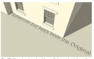
Fig 83. An extension should usually be set back from the original dwelling - 500mm is suggested.
