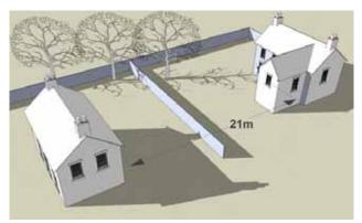
Fig 79. To protect privacy of occupants, 21 metres hould usually be allowed between primary facing windows.
