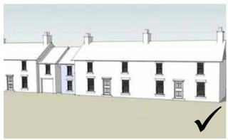
Fig 89. A preferred approach to extending would be to create subordinate extensions that maintained the primacy of the original houses.
