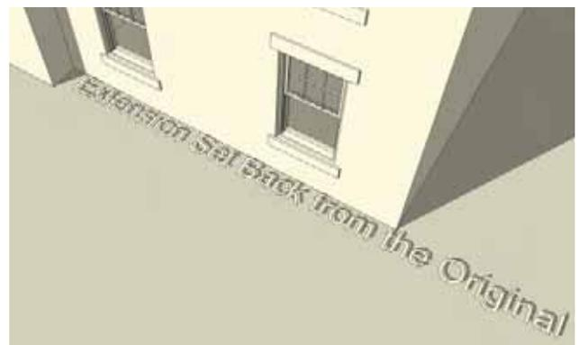
Fig 83. An extension should usually be set back from the original dwelling - 500mm is suggested.
