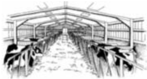
Interior of a typical modern farm building showing shallow roof pitch and portal frame construction
