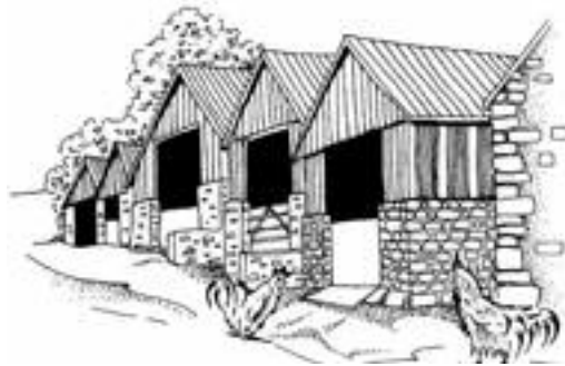
A stepped construction on a sloping site helps break up an otherwise unbroken roof line
